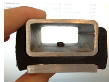
Figure F-8: A rectangular shape is more difficult to cut than a circular cross-section
