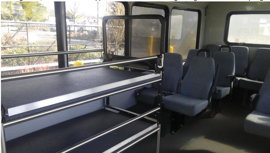
Figure 26, Interior of the Shopper Shuttle Vehicle Showing Storage Areas for Grocery Bags
